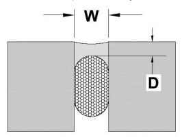
EXPANSION JOINTS - The minimum width and depth of any sealant application should be  $1/4" \times 1/4"$  (6 mm x 6 mm). The depth (D) of sealant may be equal to the width (W) of joints that are less than 1/2" wide.
