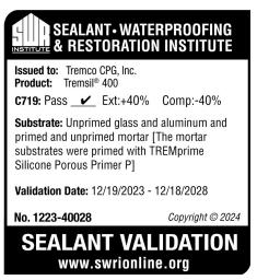
The medium modulus of Tremsil 400 grants it the capability to handle up to 40% expansion and contraction, making it ideal for use in dynamically moving joints. Tremsil 400 offers primerless adhesion to most construction materials to reduce installation times.
