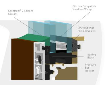
Complete glazing restoration systems from Tremco are available for a variety of applications. For the pressure bar system shown here, the original exterior gasket was replaced with Tremco's Silicone Compatible Headless Wedge and Spectrem 2 Silicone cap bead. Contact your local Tremco field representative or our Design Engineering Group for more information on our custom solutions.
