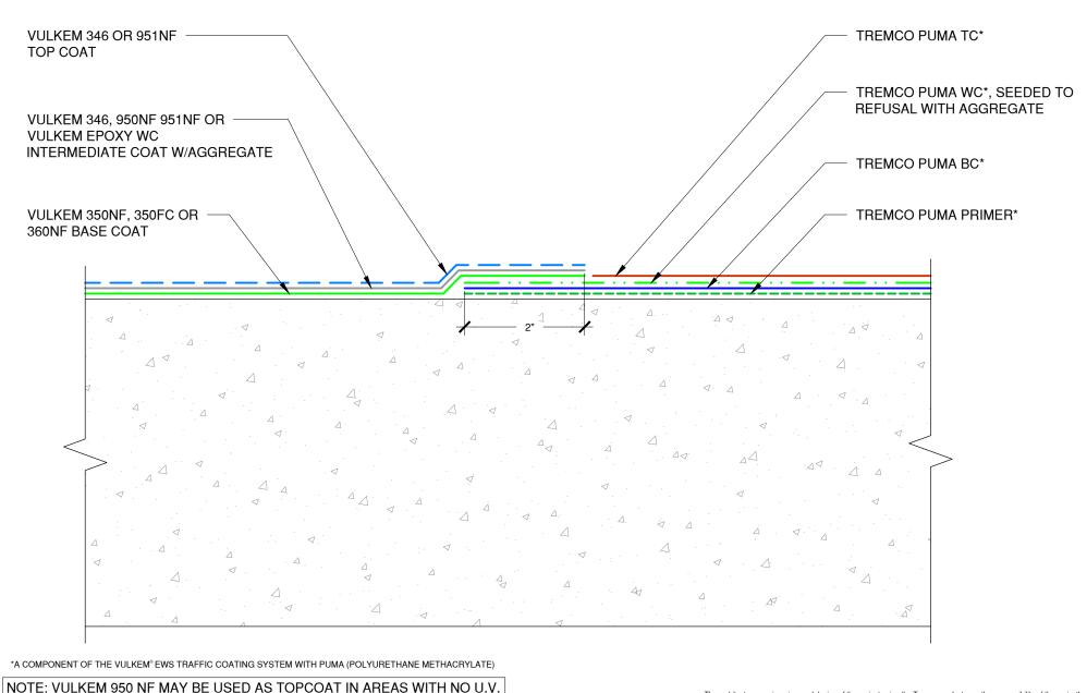
VULKEM EPOXY WC MUST NOT BE USED WITH VULKEM 350FC
