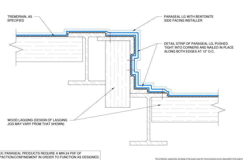
NOTES: PARASEAL PRODUCTS REQUIRE A MIN 24 PSF OF COMPACTION/CONFINEMENT IN ORDER TO FUNCTION AS DESIGNED.
