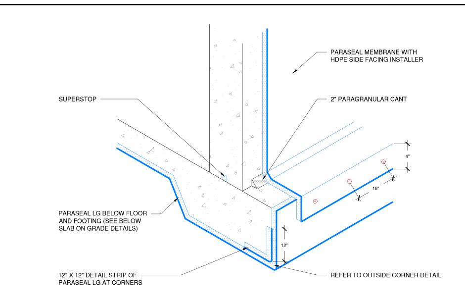
NOTE: PARASEAL PRODUCTS REQUIRE A MIN 24 PSF OF COMPACTION/CONFINEMENT IN ORDER TO FUNCTION AS DESIGNED
