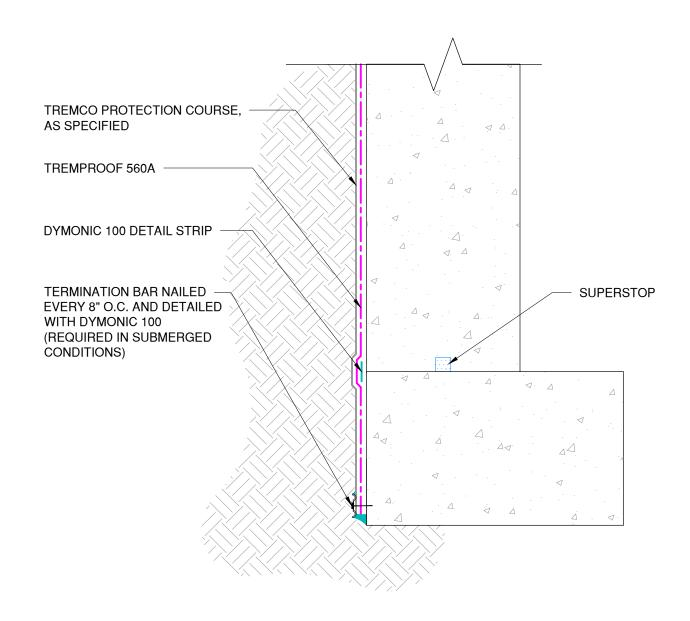
NOTE: TREMPRIME 500 MUST BE APPLIED BEFORE THE APPLICATION OF TREMPROOF 560A
