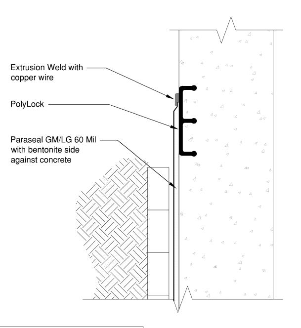
Note: Paraseal products require a minimum 24 psf compaction/ confinement in order to function as designed
