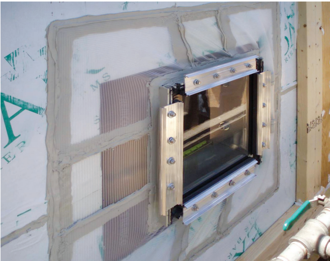
Racking wall system, seismic simulation testing (2 inches – 3 cycles)
