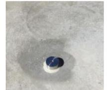
Figure 2 - A dolly bonded to substrate with Vulkem PUMA Primer
