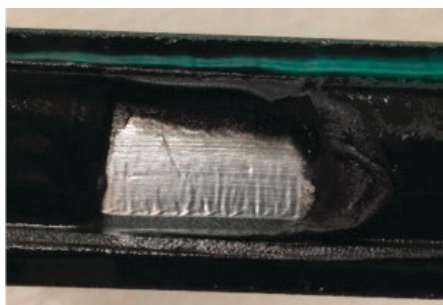
Step 3b – Hot melt removed to vapor barrier
