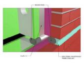
For installation of the ExoAir 111 sheet applied membrane, a bellow will need to be installed in order to account for the movement. The sheet membrane will need a bellow that is 1.5 times longer from Point A to Point B than the gap/joint width. For instance, a ½" (12.7 mm) joint would need a bellow in the sheet approximately ¾" (19 mm) long from Point A to Point B.
