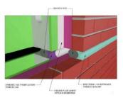
Tool sealant prior to installation of the ExoAir air barrier membrane. For installation of the ExoAir sheet applied membranes, a bellow will need to be installed in order to account for the movement. The sheet membrane will need a bellow that is 1.5 times longer from Point A to Point B than the gap/joint width. For instance, a ½" (12.7 mm) joint would need a bellow in the sheet approximately ¾" (19 mm) long from Point A to Point B.
