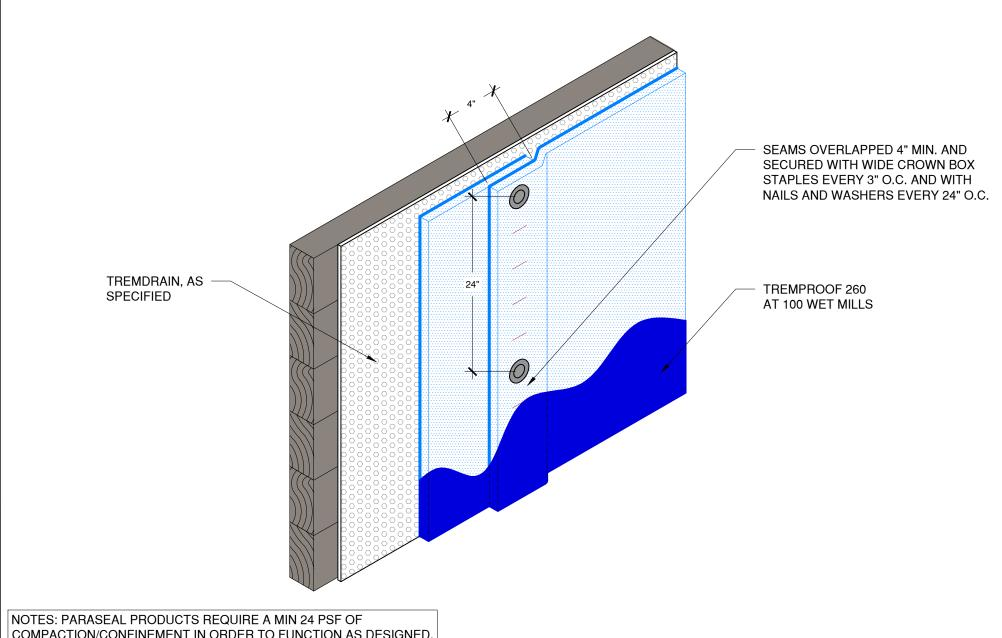
COMPACTION/CONFINEMENT IN ORDER TO FUNCTION AS DESIGNED.
