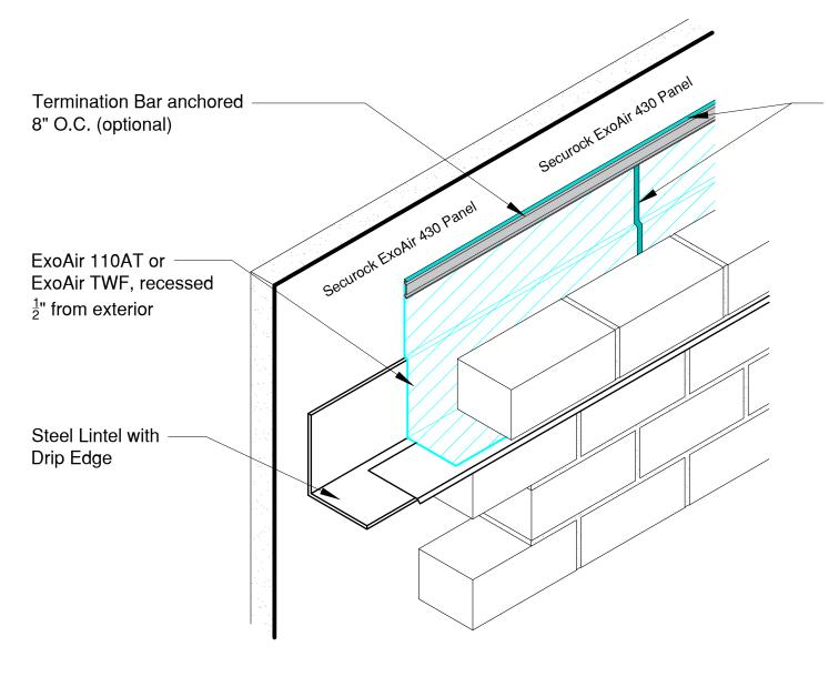
Apply Dymonic 100 to top and all cut edges of ExoAir 110AT or ExoAir TWF
