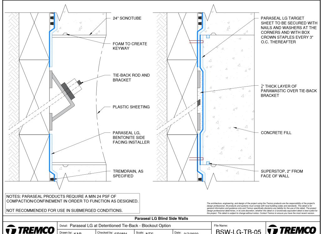
BSW-LG-TB-05 Drawn by: KAB Checked by: SP/WH Scale: NTS Date: 3/7/2022 Construction Products Group Tremco Technical Support: 866-209-2404 www.tremcocpg.com
