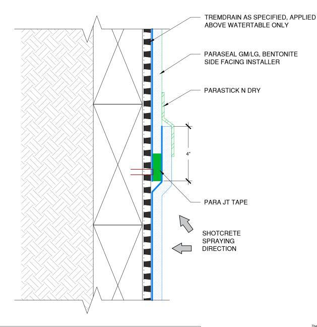
WHEN SPRAYING SHOTCRETE OR OTHER MATERIALS AGAINST PARASEAL GM/LG, SPRAY EITHER DIRECTLY AT THE SEAM OR AT THE CLOSED EDGE OF THE SEAM SO AS NOT TO LODGE SPRAYED MATERIALS BETWEEN THE LAPPED SHEETS. NEVER SPRAY INTO OPEN EDGE OF SEAM.
