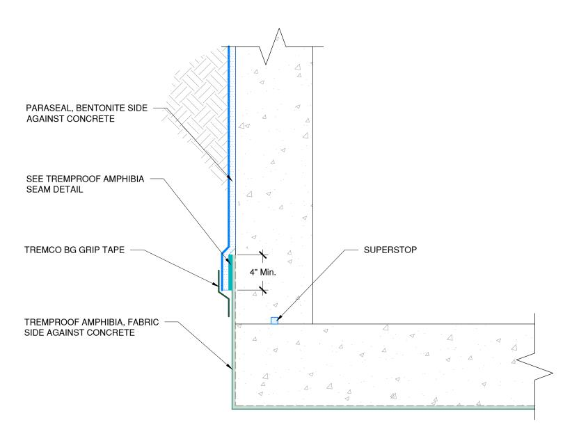
NOTE: PARASEAL PRODUCTS REQUIRE A MIN 24 PSF OF COMPACTION/CONFINEMENT IN ORDER TO FUNCTION AS DESIGNED
