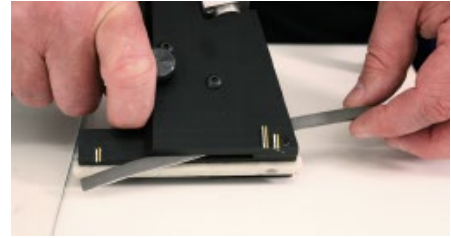
Feeding spacer through inside notching tool
